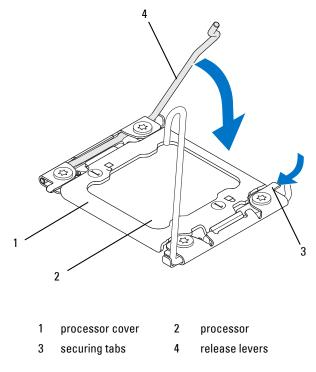
**5** Pivot the release lever down and place it under the tab on the processor cover.
